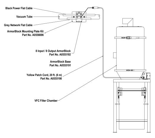
2. Attach the other connector to the **lower right** terminal of the ArmorBlock you used to connect the vacuum pump. Tighten the cord grip ring until snug.
